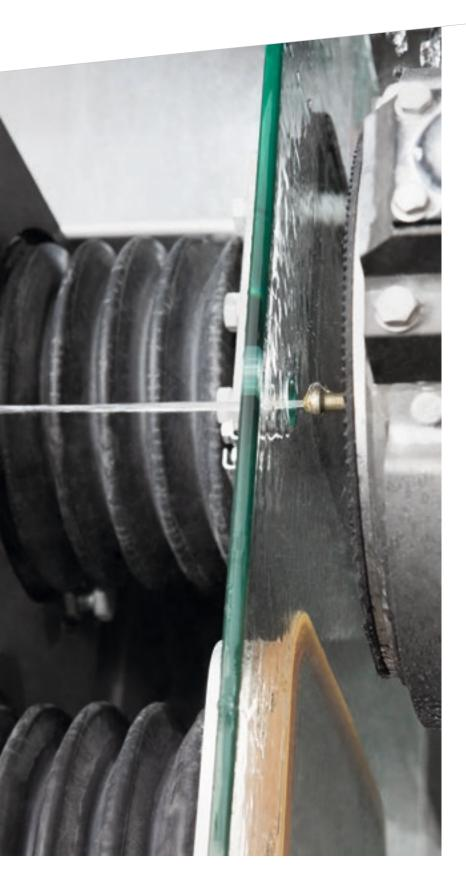
Helix is the Diamut tool that, when combined with Biesse software, exceeds all the limits of the traditional drilling systems, using one single tool for all the boring and countersinking operations on glass sheets of up to 19mm.
