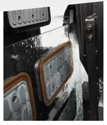
Intermac Multi Pro can easily carry out drilling, countersinking and milling operations; the complete version of the machine also allows grinding, polishing and arrising operations on the sheet edge, with the addition of a specific optional extra.
