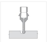
1\_Drilling with helical movement
