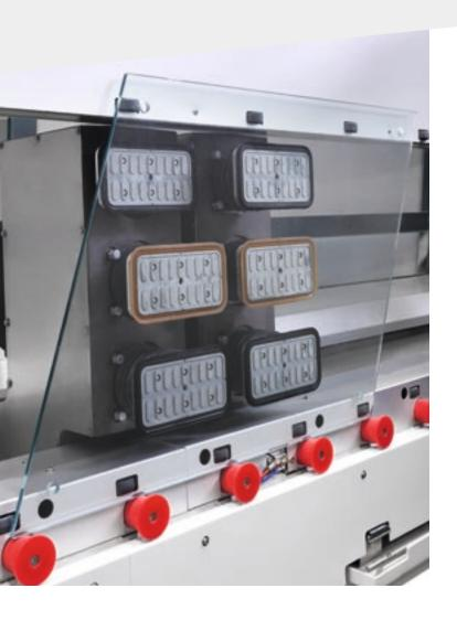
The patented dynamic repositioning system for the suction cup carriages is designed to process a piece without ever leaving it halfway between one suction cup carriage position and the next.
