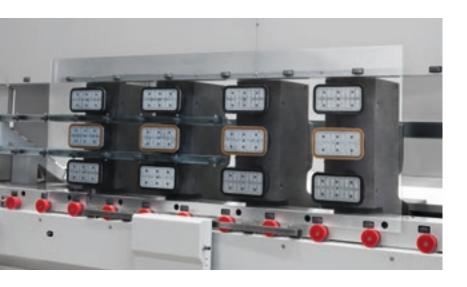
Patented system with 4 fully-independent suction cup carriages, each with 3 suction cups, guaranteeing maximum production flexibility and quality thanks to the optimised vacuum hold on the entire surface to be machined.
