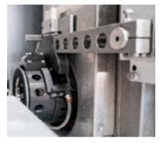
Dressing stick for dressing diamond grinding wheels and grinding device for polishing wheels.
