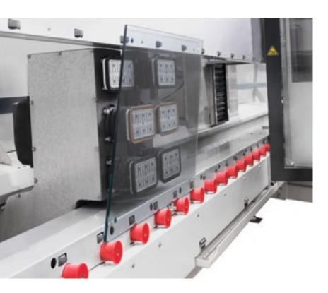
The motorised roller system allows the glass to be loaded at any point, so that the machine can begin to work completely automatically.
